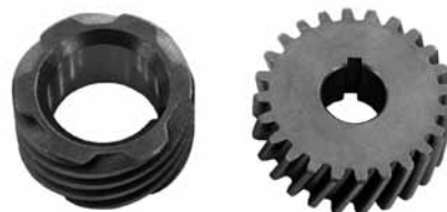
Oil Pump Gear Set Overdrive oil pump gear set includes 24T drive gear and a pinion shaft drive gear. Stock ratio for Shovelhead and Evolution models. Doubles the oil pump speed on Panhead. Fits FL and FX 1973-84. 30117
